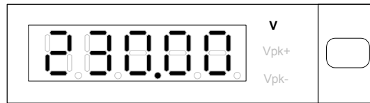
Figure 4-5 AC Voltage Display of 66201/66202 Power Meter
